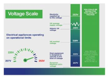
To simplify the market for electrical equipment, the European Union has introduced the Low Voltage Directive (LVD) 2006/95/EC to regulate the operating voltage of electrical equipment to be supplied in Europe. Equipment that meets the standard bears the CE mark and is designed to operate within harmonized voltage levels.
